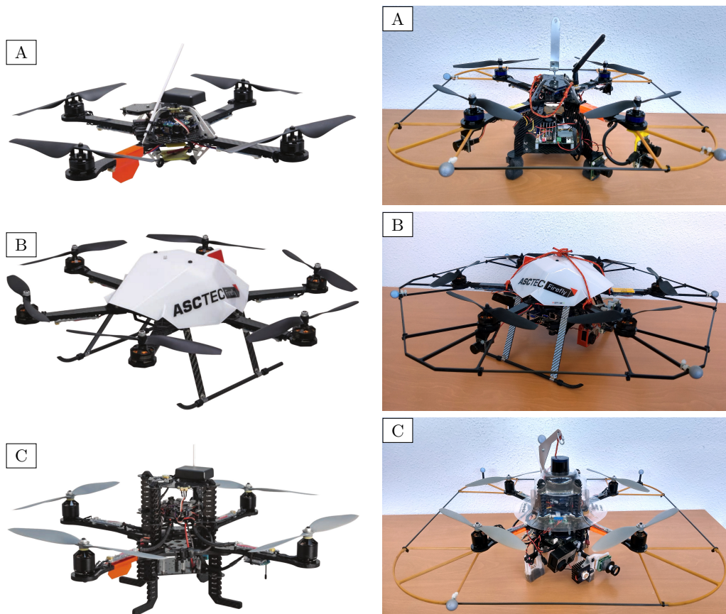
Figure 10: (Left) The aerial platforms as delivered by the manufacturer: (A) Hummingbird, (B) Firefly, and (C) Pelican. (Right) the platforms equipped with the sensor suites, on-board computers and cameras.
