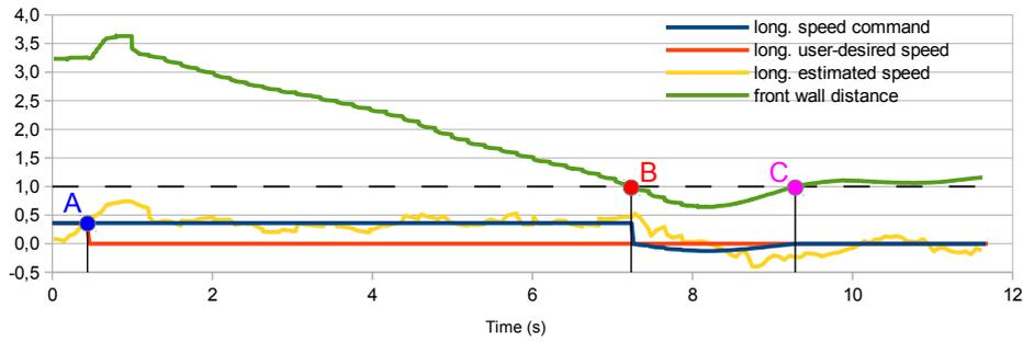
Fig. 7. Performance of the *go\_ahead* and the *prevent\_collision* behaviors: the user-desired speed is sustained while the wall is at enough distance (A→B), it is cancelled and even forced to be negative to prevent an imminent collision (B→C) until the platform is again at the safe distance (C→). All units are in SI (m or m/s accordingly).
