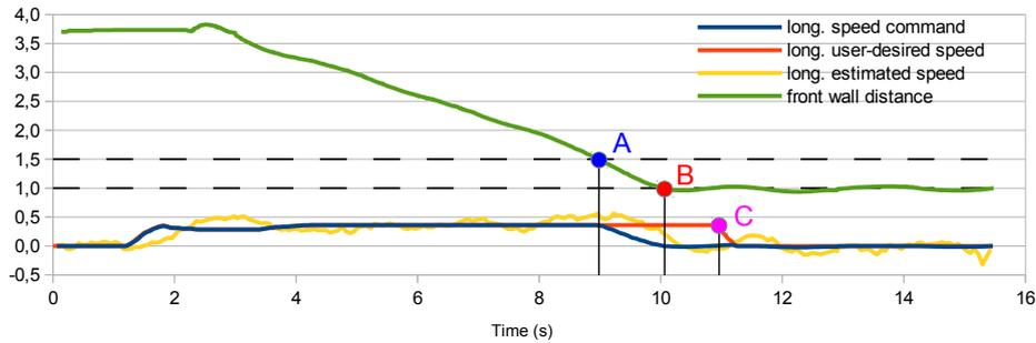
Fig. 6. Performance of the *attenuated\_go* and the *prevent\_collision* behaviors: the user-desired speed is obeyed ( $\rightarrow A$ ), it is attenuated ( $A \rightarrow B$ ) and cancelled to prevent an imminent collision ( $B \rightarrow C$ ) until the user-desired speed does become zero ( $C \rightarrow$ ). All units are in SI (m or m/s accordingly).
