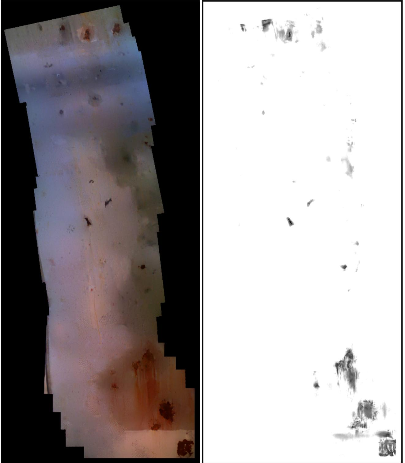
Fig. 14. Visual inspection performance: (left) mosaic built from images collected by the MAV [contrast tuned for visualization purposes], (right) defect detection result [darker pixels are likelier to correspond to defects].
