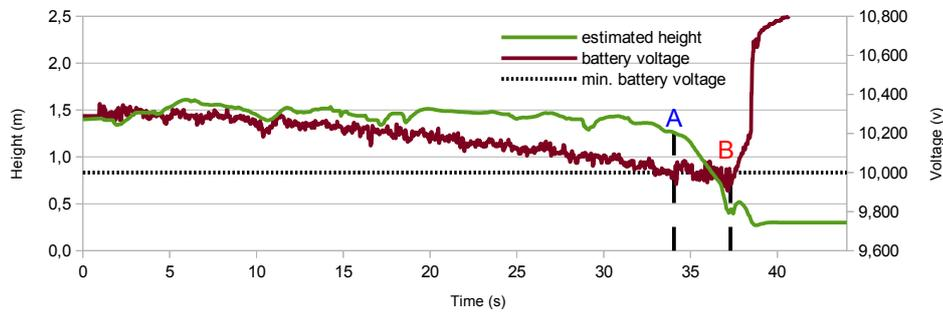
Fig. 10. Performance of the *low\_battery\_land* behavior: the platform hovers at 1.5 m until the battery voltage is below 10 V ( $\rightarrow$ A), what makes the behavior initiate the descending (A $\rightarrow$ B) and landing manoeuvres (B $\rightarrow$ ). All units are in SI (m or m/s accordingly).
