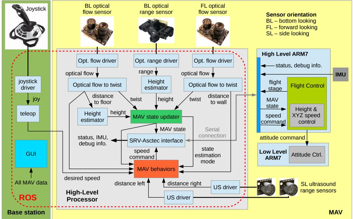
Fig. 2. Full system control architecture.
