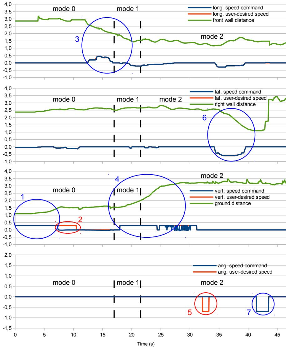
Fig. 12. Illustration of the performance of the *ensure\_reference\_surface\_detection* behavior (II): see text for the explanation. All units are in SI (m or m/s accordingly).
