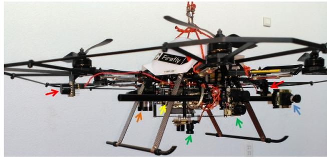
Fig. 1. Firefly platform and the visual inspection sensor suite: (green) front-looking / bottom-looking optical flow sensors, (red) left / right ultrasound sensors, (orange) height sensor, (yellow) embedded PC, (blue) camera.
