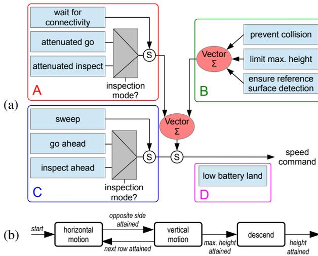
Fig. 4. (a) Behavior-based upper control layer. (b) Sweep behavior.
