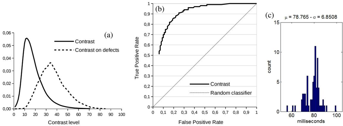
Fig. 2. (a) PDFs for contrast. (b) ROC curve for the defect detector [AUC = 0.88]. (c) Execution times.
