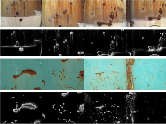
Fig. 3. Original images and corresponding defect maps.
