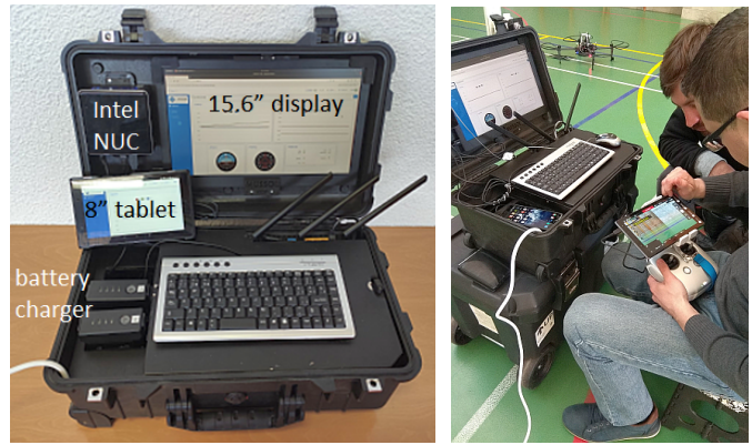
Fig. 1. The Base Station to operate the platform. (Left) Ground Control Unit (including an Intel NUC computer, a 15.6 inch. screen, a keyboard and mouse, a dual-band router and three battery chargers) and a tablet PC showing the GUI. (Right) A human operator using the base station and providing commands to the MAV through the remote controller.
