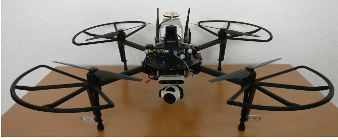
Fig. 2. Overall view of the aerial platform
