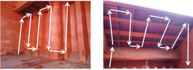
Fig. 4. Example of paths which are to be followed by the MAV to ensure an adequate level of coverage of the structure under inspection.
