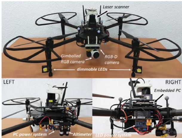
Fig. 2. ROBINs aerial platform, fitted with a laser scanner, a height sensor; a camera set featuring LED-based illumination, and an embedded PC.
